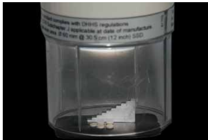
2 Radiographic unit and image plate.
